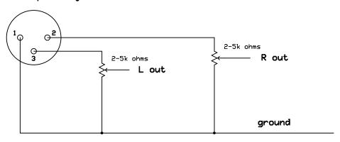
The Cue amp is a power amp. Be careful to not short the outputs to ground or power rails!
